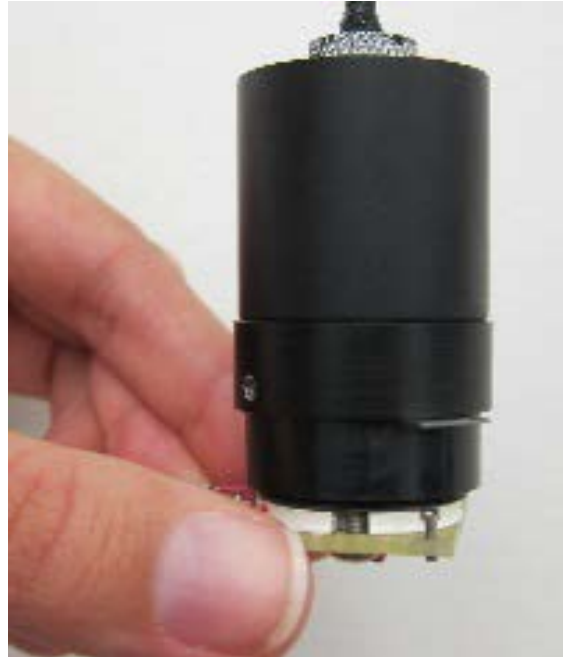
Figure 3.1 Photograph of the deep-UV LED detector.
